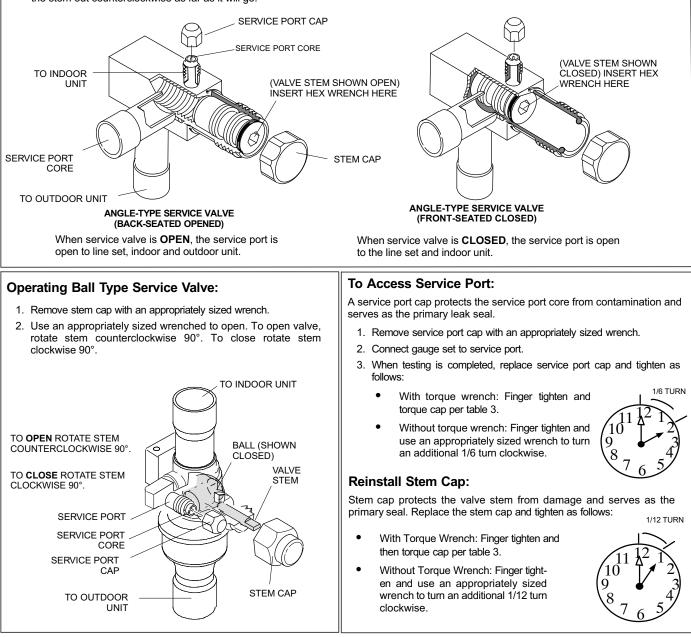
NOTE — A label with specific torque requirements may be affixed to the stem cap. If the label is present, use the specified torque.
